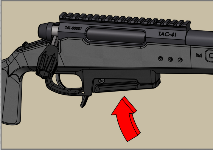
Engage a loaded magazine to pre-fill the feeding ramp (20 bbs are required).
