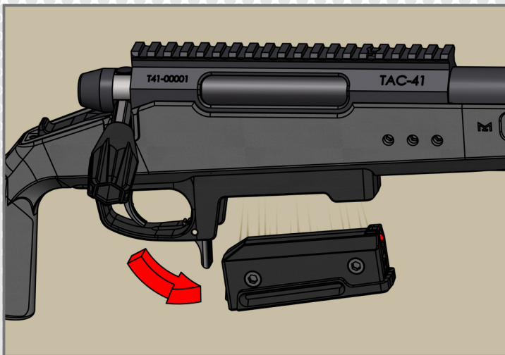
Disengage the magazine.
