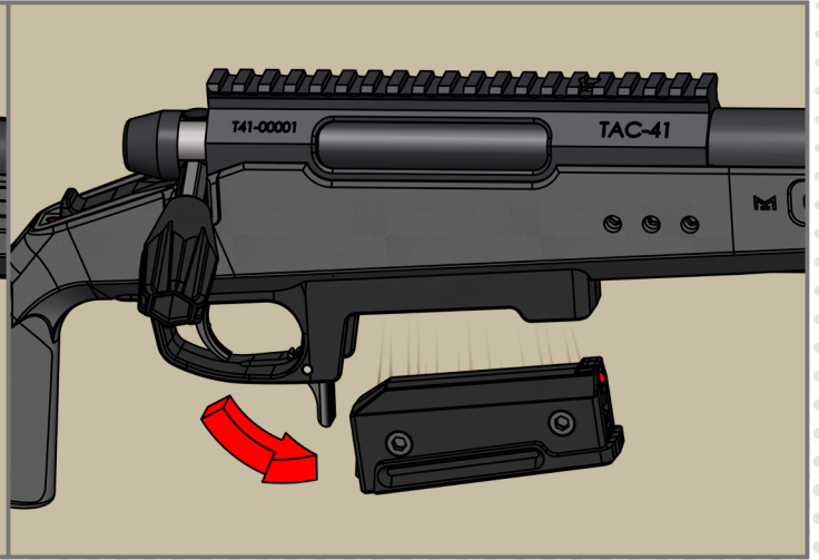
Disengage the magazine.
